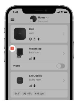
If a malfunction is detected in WaterStop (for example, there is no connection with the hub or range extender), the malfunction counter is displayed in the device field in the Ajax app.
